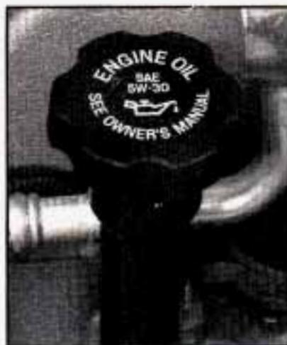
The engine oil fill cap for the 4.3L, 5.0L and the 5.7L engine is located on the driver's side engine valve cover.
