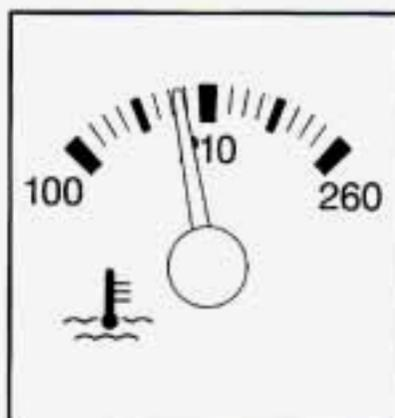
This gage shows the engine coolant temperature.
