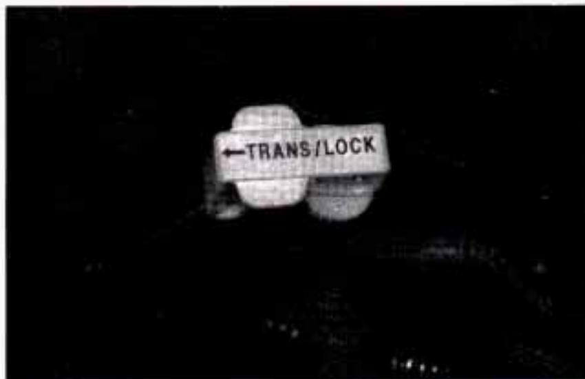
The red transmission dipstick handle is located at the rear of the engine compartment, on the passenger side.
