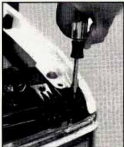
1. Remove the two screws at the top of the radiator support.
