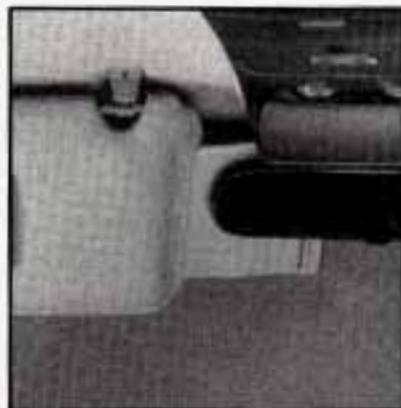
Some visors have an extender on the inside edge. When the visor is down, pull the extender out for extra glare coverage at the front or side.
