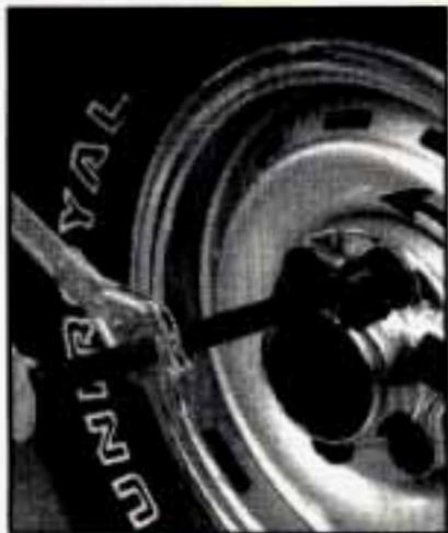
If your vehicle has wheel nut caps, use the wheel wrench and ratchet to remove them. Turn the wheel wrench counterclockwise, with DOWN facing you, to remove the wheel nut caps.
