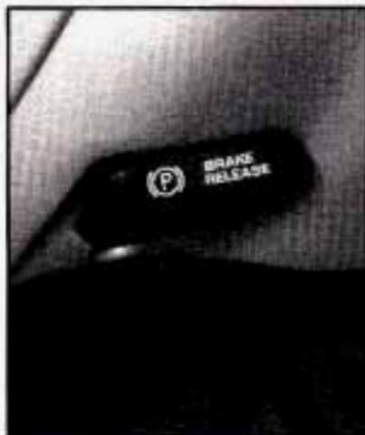
Pull the lever, located just above the parking brake pedal, marked **BRAKE RELEASE**.
