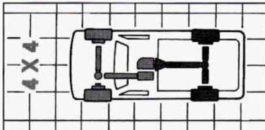
The front axle portion of the indicator diagram will light up when you shift into four-wheel drive.
