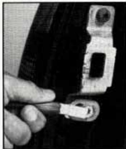
1. Raise the tailgate slightly and release both retaining cable clips. To release the cable clips, lift the cable so it points straight out and push the cable clips forward.
