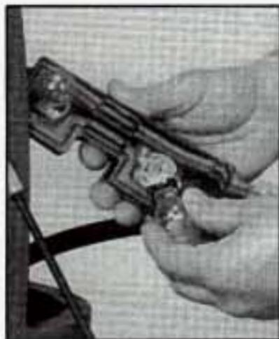
4. Pull the old bulb straight out of the socket.
