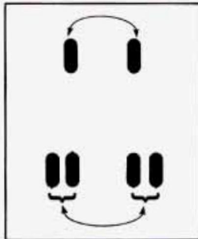
If your vehicle has dual rear wheels and the load range or tread design for your front tires is different from your rear tires, always use the correct rotation pattern shown here when rotating your tires.
