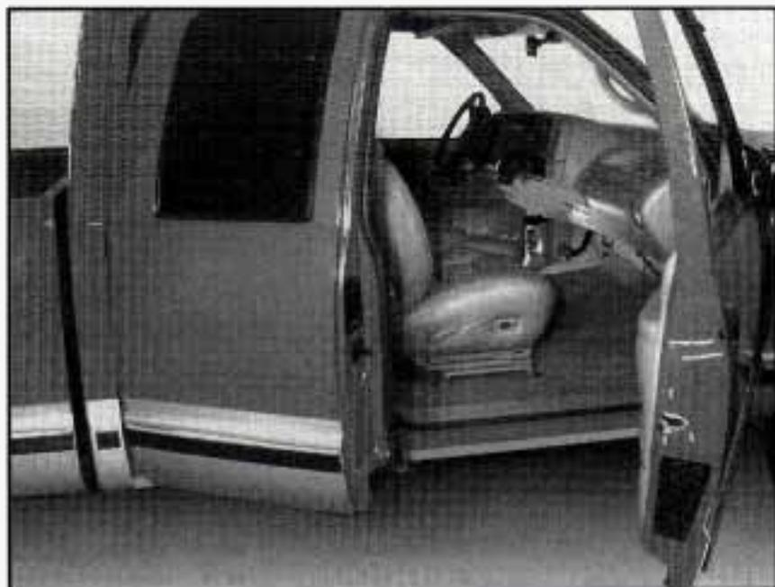
Your vehicle may be equipped with a third door that allows easier access to the rear area of an extended cab.
