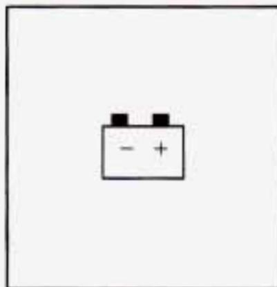
This light should come on briefly when you turn on the ignition, before starting the engine, as a check to show you it is working.
