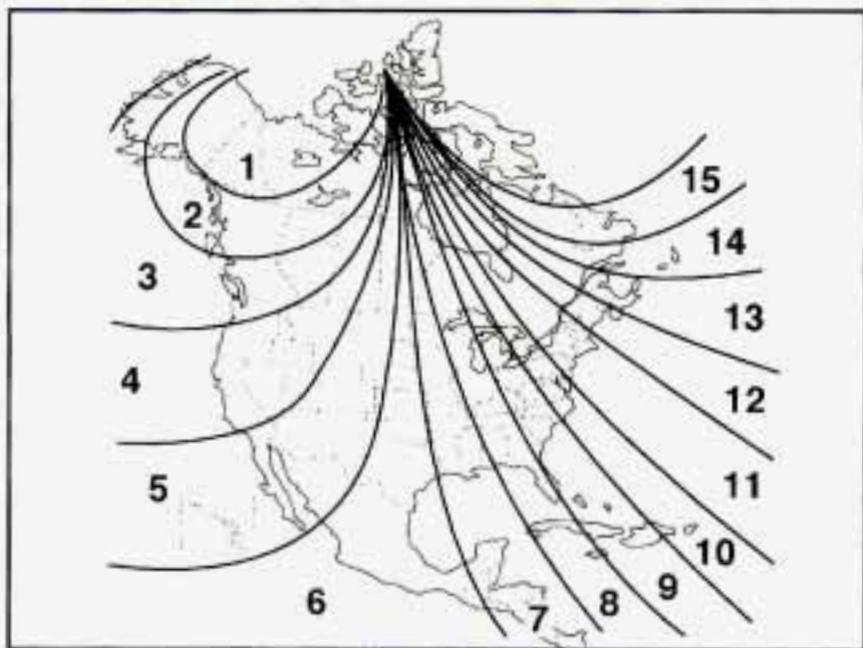
3. Press the CAL switch on the bottom of the mirror until the new zone number appears in the display. After you stop pressing the button in, the display will show a compass direction within a few seconds.
